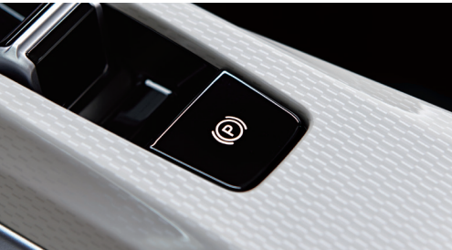
Electronic parking brake with auto-hold function
