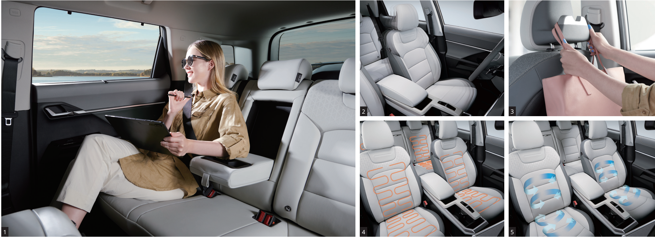
1. 40:60 split rear seats with 32.5° reclining 2. Powered 8-way front seats with driver 2-way lumbar support 3. Hanger headrest 4. Heated seats, front and rear 5. Ventilated front seats
