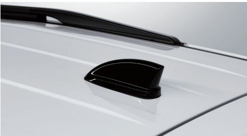
Shark-fin antenna with glonass, DAB and GSM
